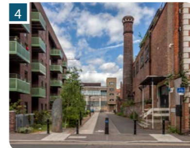
Ensuring controlled vehicle access with movable bollards to street entrances.
